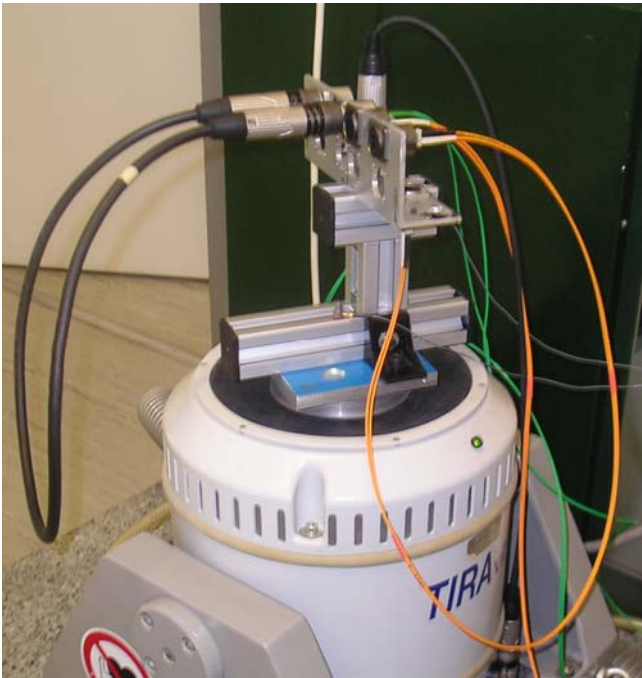
Fig. 2a: Vibration equipment and test cable arrangement
