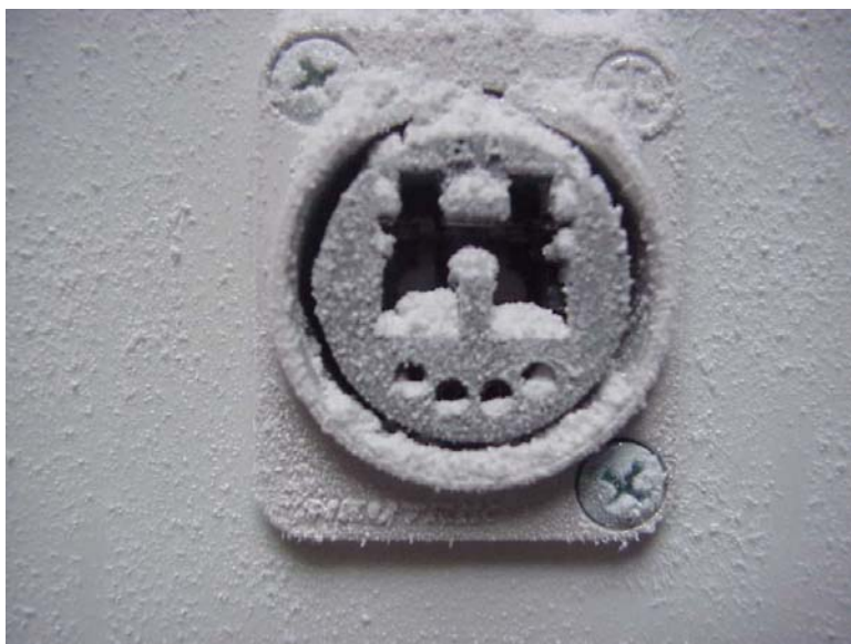
Fig. 10: Dust sediment on the front side of the receptacle after 60 min.
