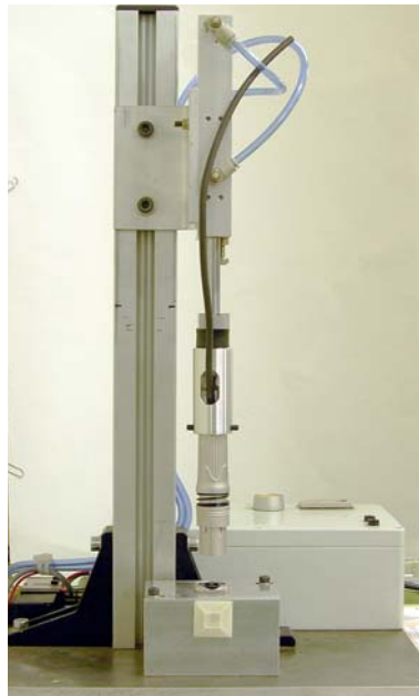
Fig. 5: Test facility for mating durability
