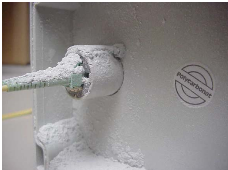
Fig. 9: Dust sediment on the rear side of the receptacle after 60 min.
